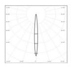
AEP5MI-65ML130BK 10° **BEAM ANGLE:** 67.81W 3858.6 lm 69891 cd 56.9 lm /W
