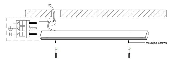
3. Install the light source module and light source profile into the light body, then lock the swivel screws with a screwdriver, and install the mask and end cap into the light body in order.
