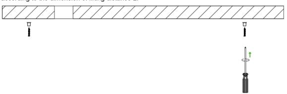
2. Secure the T-piece to the ceiling piece by tightening it.
