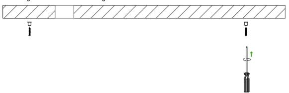
2. Secure the T-piece to the ceiling piece by tightening it.
