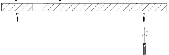
Secure the T-piece to the ceiling piece by tightening it.
