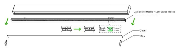
2. Connect the power input wire of the fixture to the power supply, L is the fire wire, N is the zero wire, is the ground wire, and the input voltage is AC 220V~240V 50/60Hz. Align the mounting screws with the mounting holes of the fixture, secure it with a screwdriver or a power tool, and fixed the luminaire on the ceiling.
