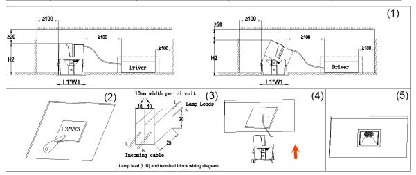
3.If the driver of the luminaire comes with its own lead, and this connection lead needs to be connected with an independent terminal block (refer to Figure (3) schematic wiring), the size of each terminal block should be not less than 10\*20\*25mm.
