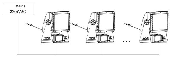
4. Dimming Version of the Wiring Diagram: Connect one end of the power input line to the utility line, then connect the dimmer line to the dimmer controller.
