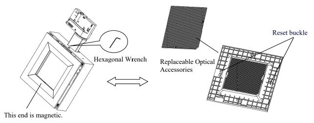
3. The installation sequence is the reverse of the removal sequence. Install the cover in the direction of the corresponding buckle, and when you hear a "click" sound and the lamp cover is not raised, it is installed.
