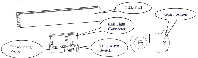
2. Align the projection of the guide rail light connector with the groove of the guide rail before assembly.
