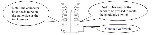
3. After assembly, turn the "Conductive Switch" clockwise by 90 degrees to conduct.
