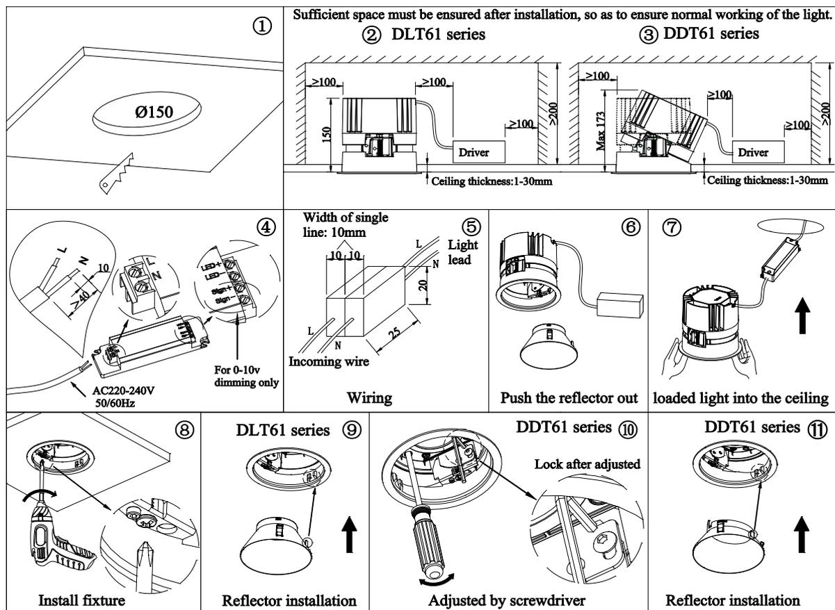
\* If the driver of the light comes with lead wires, and the leads need to be connected with an independent terminal block (refer to Figure 3 for wiring), the size of the terminal block for each line should not be less than 10x20x25mm.
