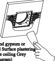
Mesh board and gypsum or wooden board Surface plastering after fixing the ceiling Grey (schematic diagram)
