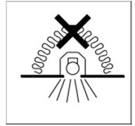
Warning: See signs. Under no circumstances should lighting fixtures be covered with insulation pads or similar materials
